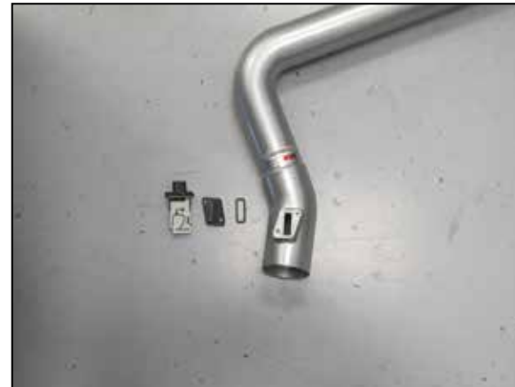
20. On vehicle equipped with a humidity sensor, install the sensor into the K&N® intake tube. On all other vehicles install the provided gasket onto the block off plate and install the block off plate onto the K&N® intake tube.
