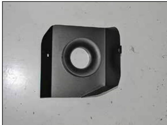
15. Install the provided filter adapter into the heat shield and secure with the provided hardware.
