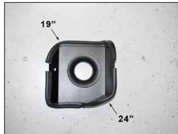
17. Install the edge trim onto the heat shield as shown.
