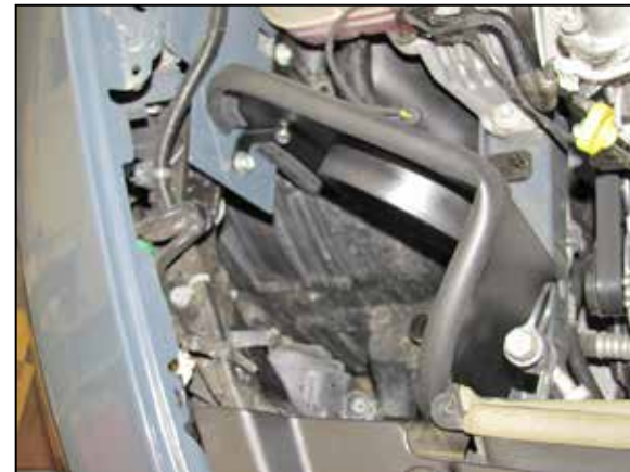
18. Install the heat shield assembly onto the brackets installed previously using the provided hardware.
