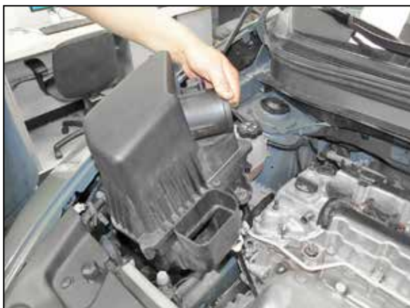
10. Lift up the air filter housing to dislodge it from the mounting grommets and remove it from the vehicle. NOTE: K&N Engineering, Inc., recommends that customers do not discard factory air intake.
